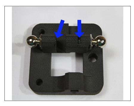
Install two ball studs using two M3
