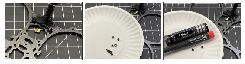
Insert M2x8 screws thru the bottom plate and thru the TPU antenna mount as shown, add nylon washer, and secure with M2 lock nut
