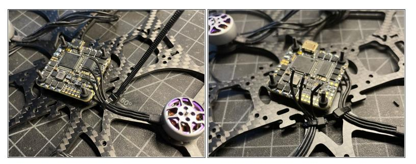
Trim motor wires, remove 2mm of insulation, pre-tin wires, and solder to motor pads
