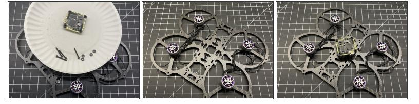
Insert M2x16 Button Head screws X4 in frame as shown and add plastic washers if needed for FC clearance.
