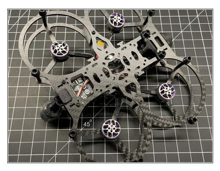
Screw the top plate to the bottom plate using M2x8mm screws
